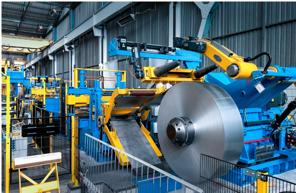
New narrow-strip center for stainless steel manufactures strips up to 25 km long (Mannheim site)
